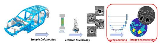
New strategies in the field of characterization and design of light-weight and sustainable materials still lack more accurate information about the statistics of microstructural details, such as where damage originates at the microscale (see image above). For this, large amount of data need to be analyzed. Computer vision as a daily growing machine learning based pipeline provides a vast horizon of opportunities in this context of materials science.
