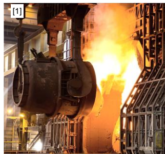
[1] Charging an LD converter POSCO, Korea
