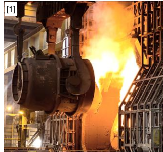
[1] Charging an LD converter POSCO, Korea
